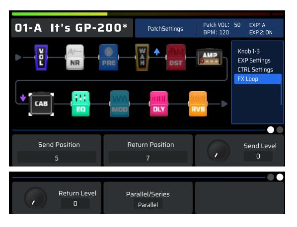
FX Loop: the FX Loop settings in the current patch. Blue arrow ↑ the signal is sent from here. Purple arrow ↑ the signal is returned here. The Send/Return nodes can be freely moved in the effect chain.
