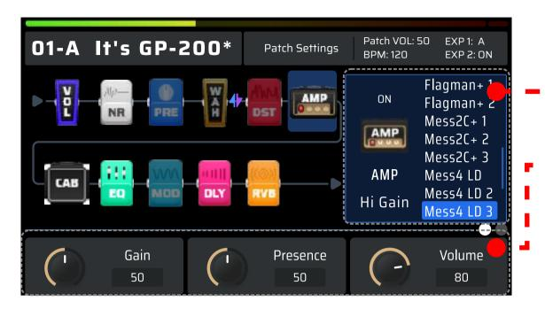
All effects in the module are listed on the right of the screen, turn PARA knob and click to switch effects.
